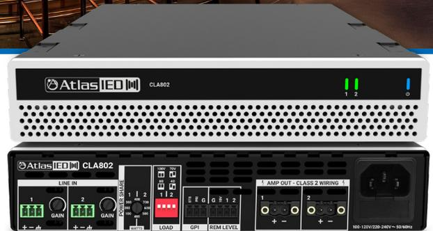
The CLA Series is a high-power amplifier designed for versatility, suitable for both commercial 25V / 70V / 100V distributed systems and professional applications requiring amplification for low impedance loads like 4Ω or 8Ω. Notably compact and lightweight compared to similar-performing models, the CLA Series incorporates an efficient Class D output topology while offering the fidelity of a Class AB amplifier.
