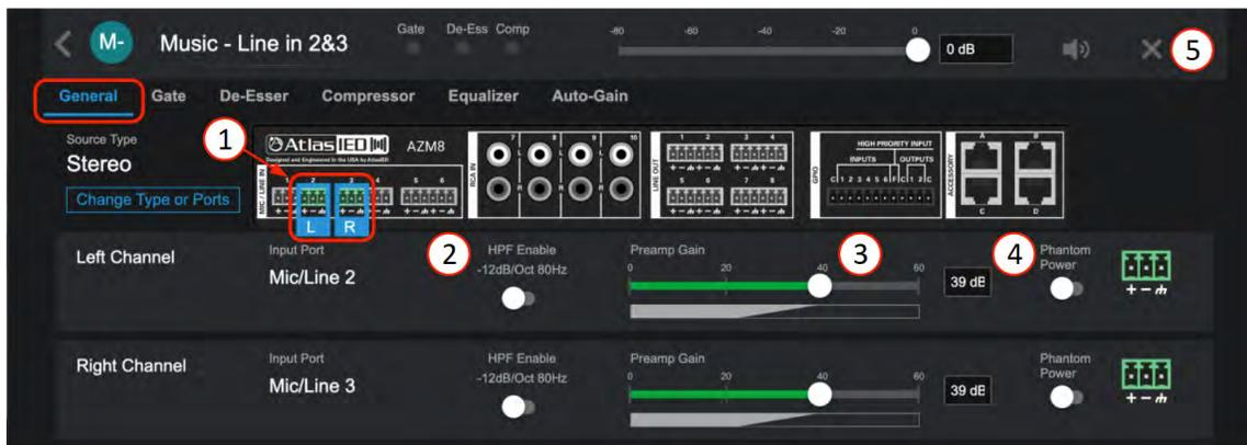
1. Mic/Line Stereo sources require selecting a Left and Right input port which can be any available Mic/Line Inputs.
