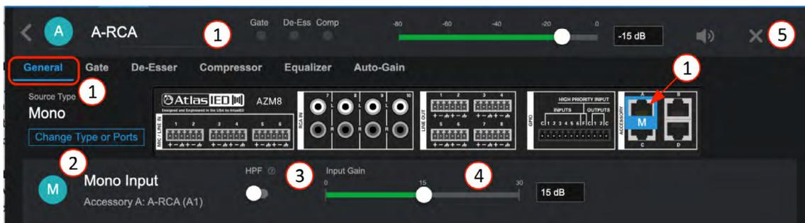
1. The General Settings page displays the editable Source Name, identifies physical location of input for wiring, and navigation tabs for DSP settings: Gate, De-Esser, Compressor, Equalizer, and Auto-Gain. (same as DSP on Mic/Line page above).
