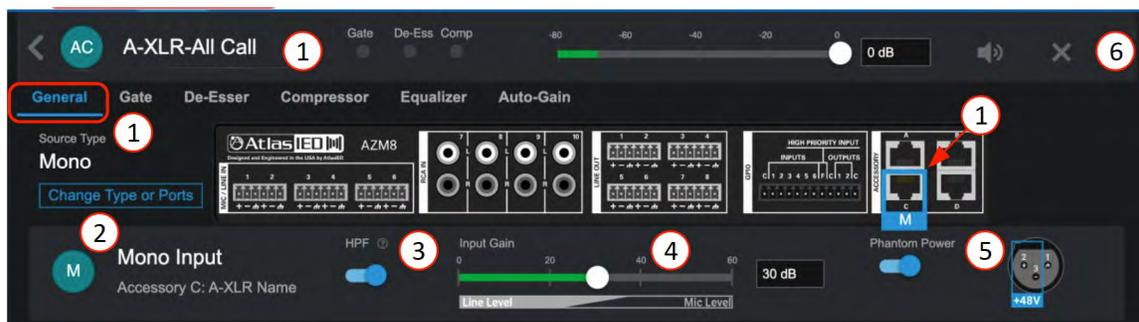
1. The General Settings page displays the editable Source Name, identifies physical location of input for wiring, and navigation tabs for DSP settings: Gate, De-Esser, Compressor, Equalizer, and Auto-Gain. (same as DSP on Mic/Line page above).
