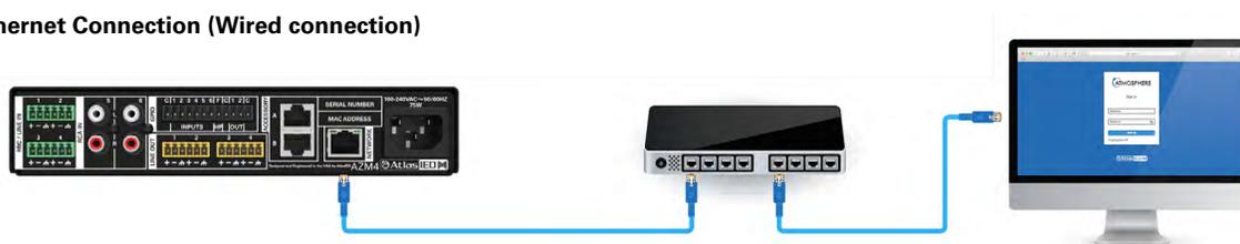
Connect an RJ45 cable (CAT5e or CAT6) from the AZM ethernet port to an existing network.
