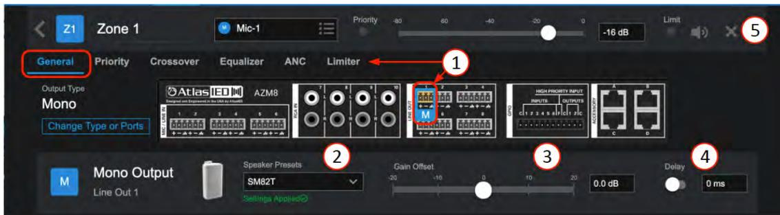
1. The General Settings page shows the port to wire connection to, and DSP settings pages for Priority, Crossover, Equalizer, Ambient Noise Compensation (ANC) Control, and Limiter.
