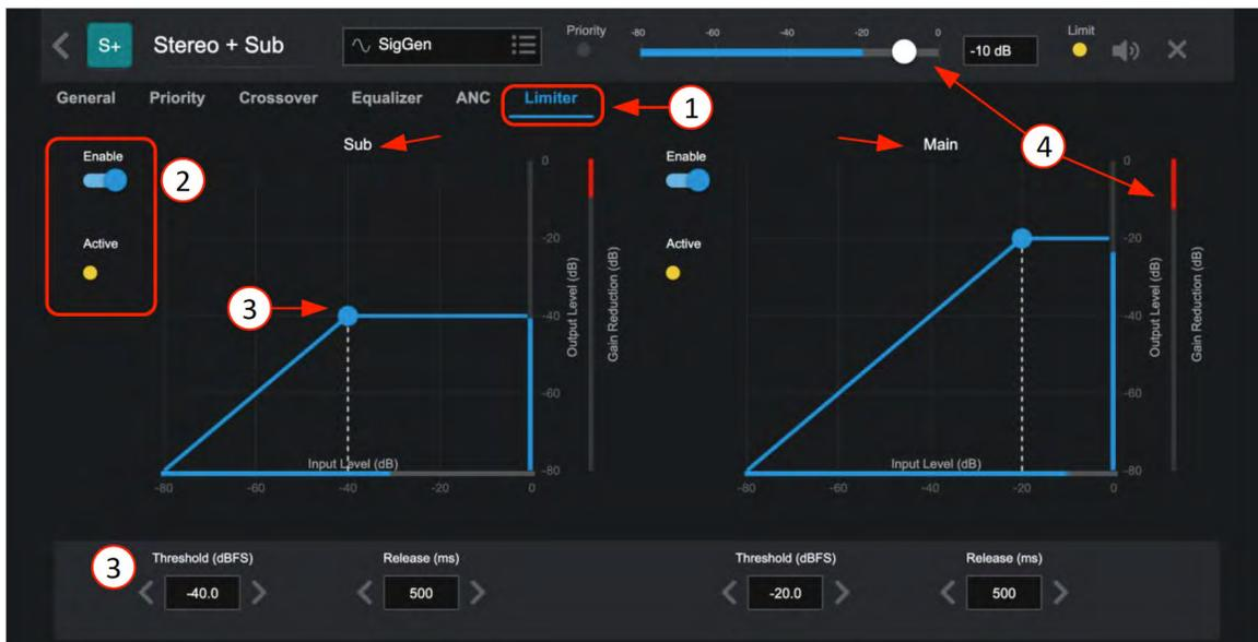
1. The Output Limiter is used primarily for taming transient peaks to keep the output signal strength below a specified level. This can help prevent damage to loudspeakers in the event of unintended loud signals like the drop of a microphone. When Zones are Mono or Stereo, only the Main Limiter is displayed. When a Sub is added, a separate limiter is available to tame the energy of the Sub so it doesn't affect the Main.
