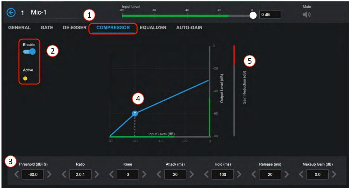
1. A compressor is a dynamic setting that can automatically reduce peaks in volume and smooth out a radically changing signal. It is used differently depending on what instrument or signal is being tamed. Compressing reduces the peak levels by squashing the sound into more even levels, reducing channel clipping, while remaining loud. A good setting sounds natural and rich. The art of setting up a compressor correctly takes some practice. While learning, subtle changes are a good routine.
