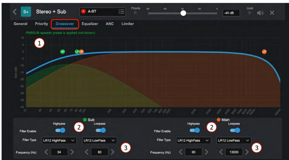
1. The Crossover provides a HighPass and LowPass adjustable filter for Main (Mono and Stereo source) and when Sub is added, an additional HighPass and Lowpass just for the subwoofer. Dynamically move graphic or select and enter settings.
