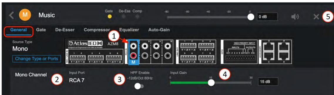
1. Displays rear panel and identifies physical location of the RCA mono-summed input for wiring. Navigation tabs for Gate, De-Esser, Compressor, Equalizer, and Auto-Gain. (same as Mic/Line).
