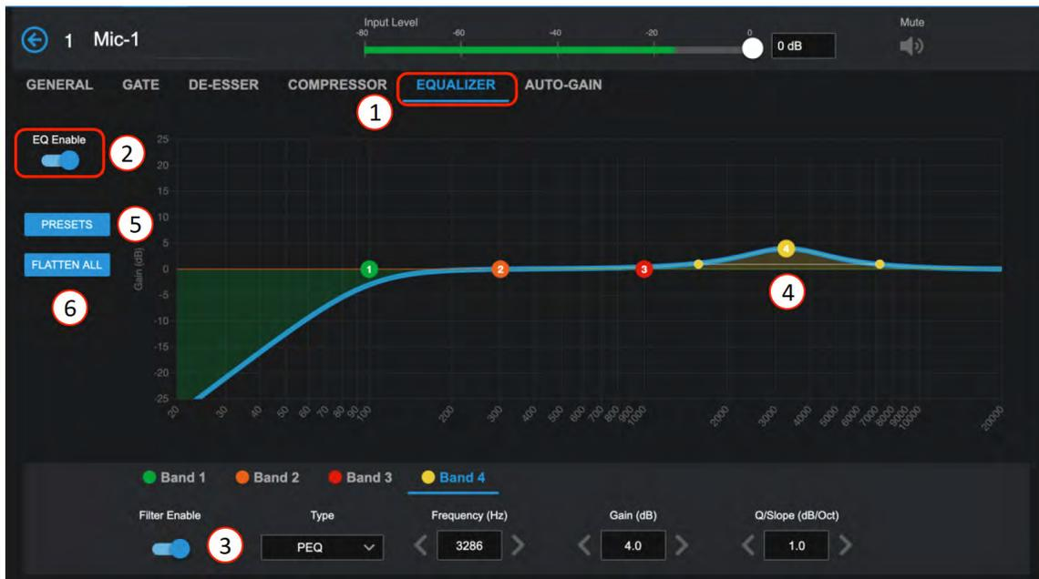
1. Equalizers allow raising or lowering the level of individual frequencies or ranges (bands) of frequencies to improve the overall sound of a source signal. Narrow bands can also be set to remove problems, like feedback or an acoustically induced low end.
