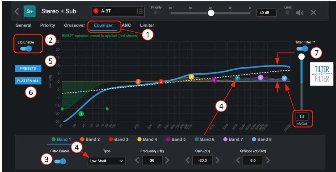
1. Equalizers allow raising or lowering the level of frequencies or ranges (bands) of frequencies to improve the overall sound of a source signal. Narrow bands can also be set to remove problems, like feedback or an acoustically induced low end.
