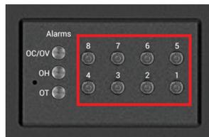
**Alarm Indicators** - The AP-IP power distribution systems feature alarms for the following: Over & Under Voltage, Over Current, Over Temperature and Over Humidity. All alarm settings are programmed in the web UI. If an alarm is activated, the associated LED will illuminate and the fault contacts will open.
