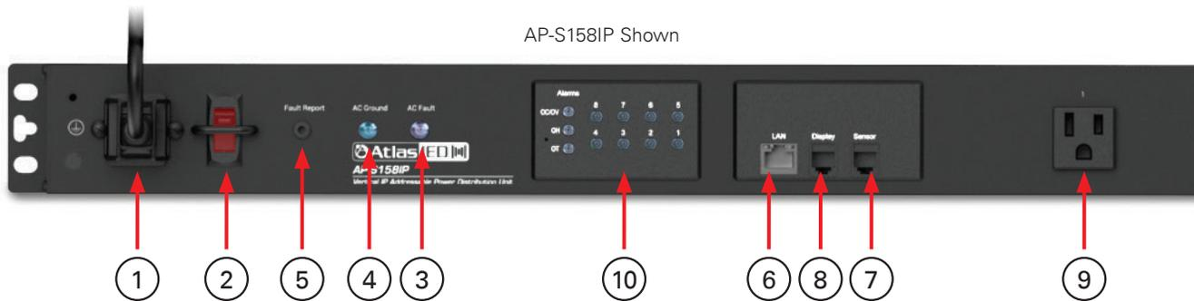
1. **AC Mains Input** - Connect the IEC 14-Gauge 6' (2m) power cord to a 15A 120VAC outlet to provide power to the unit. An IEC power cord retainer clip is included to prevent accidental removal of the power cord from the unit.
