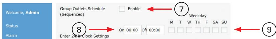
7. **Grouped Outlet Scheduled (Sequence) Enabled Button** - When this box is checked all outlets assigned to the Grouped Outlet will be sequenced On / Off at the time and days entered.
