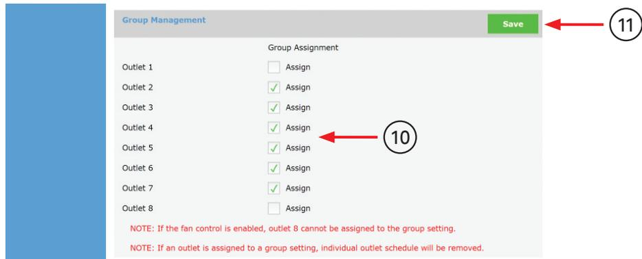
10. **Group Assignment** - Each outlet can be assigned to a Group to be sequenced On / Off.
