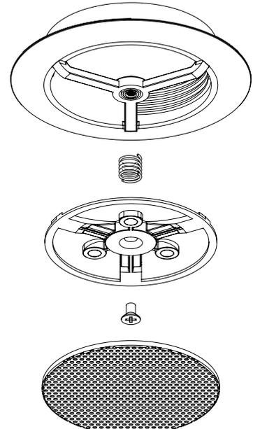
Direct Fire Lens (4mm) with Direct Fire Grille
