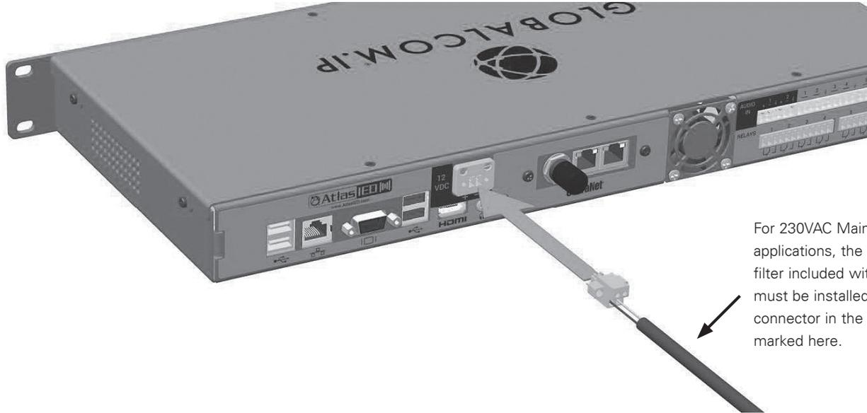
For 230VAC Mains applications, the ferrite filter included with the unit must be installed near the connector in the vicinity marked here.
