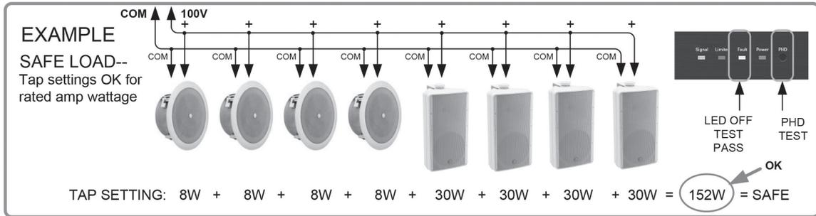
The Fault LED should never be constantly illuminated or damage may occur to the amplifier or sound system. If the Fault LED comes on steadily during use or during the PHD test there are a few common fault conditions to check if using a 100V distributed audio system.
