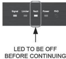
**Note: During the initial start of the diagnostic test, the Fault indicator may flash Yellow for a few seconds until an accurate diagnostic reading has been completed, continue to hold the PHD switch in for 5 seconds to assure the test is complete. After 5 seconds and the Fault indicator is illuminating Yellow steadily, stop and read the section "How to Trouble Shoot Your Speaker System If the Fault LED is Illuminating."**
