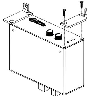
4. **TSD-RMK Optional 19" Width Rack Mount Kit** - For 19" rack mounting, Atlas Sound offers an optional rack mount kit, the TSD-RMK. This rack mount kit can support up to four TSD units. The kit includes three blank panels designed to fill any unused slots. Use the included hardware to mount the TSD into the rack mount kit using the top mount screw holes on the TSD.
