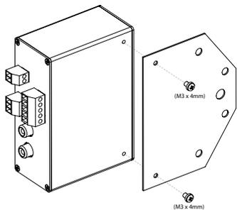
3. **Panel Mount Brackets** - Atlas Sound offers an optional set of "L" mounting brackets. Remove two of the screws from the front panel, align with the holes on the brackets, and secure the screws to install. The brackets are not identical; there is one for the Right and one for the Left.
