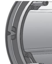
Grille tabs aligned with notches on the unit bezel
