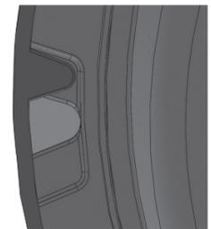
Grille tabs secured to the unit bezel
