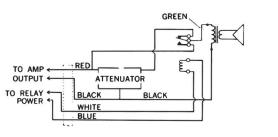
Wiring Requirements: (1) Pair for Audio, (1) Pair for Relay
