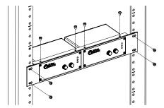
3. TSD-RRMK Rear Rack Mounting Kit - For complete flexibility in mounting a TSD or TSD external power supplies the optional TSD-RRMK is available. The TSD-RRMK can support mounting of either two larger TSDs with external power supplies or up to 4 TSD models. Note: Only use the included M3 x 4mm screws as other screws may be too long and will cause internal damage to the TSD.
