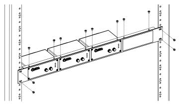
TSD-RMKHR Half Width Rack Mount Kit - AtlasIED offers an optional rack mount kit that can be used in half width rack applications including the AtlasIED WMA-HR and AWR-HR models. The TSD-RMKHR can support up to two TSDs. Included is an extra blank panel to fill one of the spaces if only one TSD is being used.
