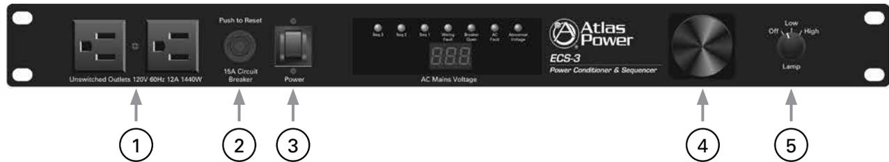
1. **Unswitched AC Outlet** – The two 120VAC outlets are always live when the ECS-3 power cord is plugged into an AC mains power source and voltage is present. If voltage is present at the outlets, it will be displayed on the AC Mains Meter.
