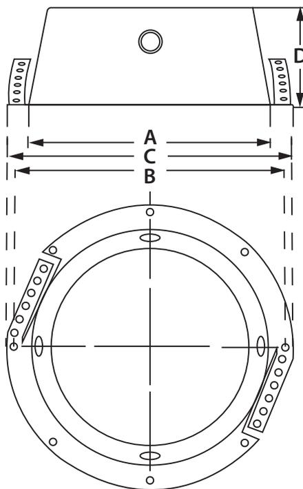
NOTE: The CS95-8 Series enclosure will mount speakers with most Atlas Sound premounted line transformers. The HT-87, HT-167, and HT-327 transformer however, will not fit the enclosure when premounted to the speaker. Please consult appropriate speaker/transformer specification sheet for dimensions.
