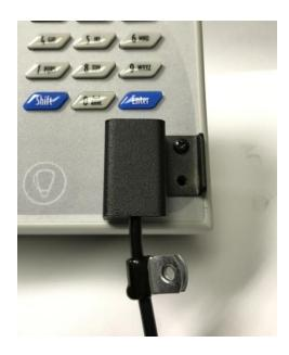
STEP 2 – Gently bend the cord down to place the new bracket over the connector. Align the two holes with the faceplate and install the #6-32x3/8" screw in the top hole to hold the bracket in place.
