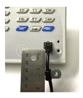
STEP 1 – Remove screw from existing strain relief clip and lower right mounting hole. Adjust clip 1" away from RJ25 plug. If no strain relief clip is present, install the included one at this location.
