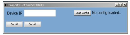
b. Input the IP address of the DNA amp frame in the **Device IP** edit box. Next, press the "Load Config" button to open a file browser. In the file browser, find and open the "DNA7800 Version Info.xml" file.
