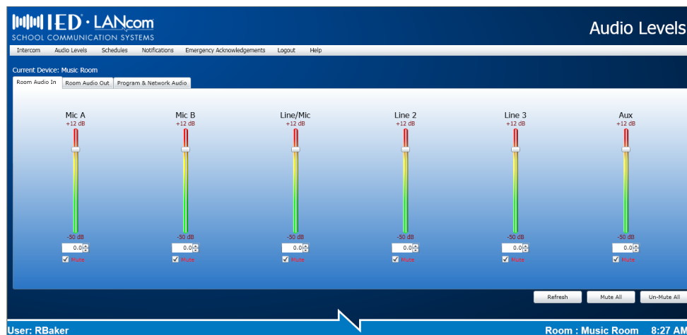
Figure 6-5: LANcom SCS User Screen - Paging Console - Room Audio In tab
