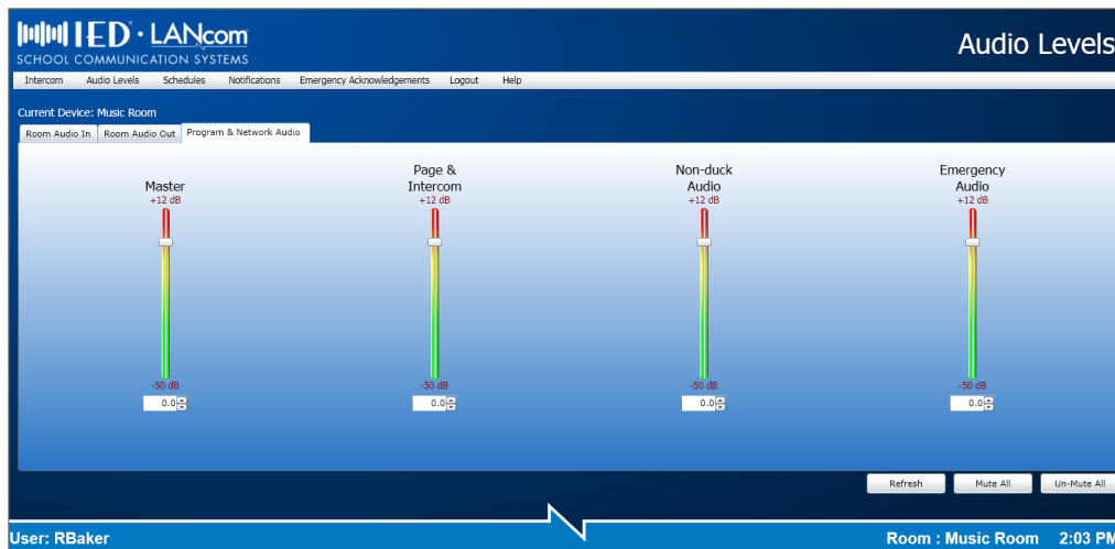
Figure 6-10: LANcom SCS User Screen - Paging Console - Program & Network Audio tab
