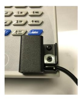
STEP 3 – Hold the strain relief clip in place over the bottom hole and install #6-32x1-1" flat head screw to secure clip. Tighten both screws to complete installation.
