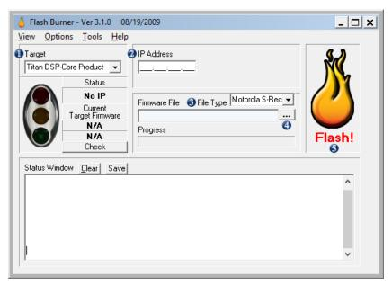
The little blue circled numbers that appear on the user interface indicate the steps to follow when using this tool. For this situation, it is useful to insert a step between ② and ③. This extra step insures that one is talking to the frame on the network and retrieves the current firmware version which is used to determine which version of the latest firmware to apply to this frame (as explained in Appendix A and listed in Appendix B).
