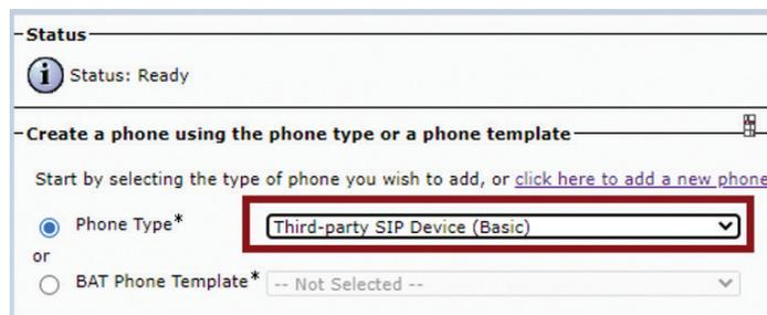
Following basic phone/end user configuration procedures, input the device MAC address in the MAC Address field and choose the desired Device Pool, e.g. 'Default'. For the Phone Button Template, select Third-Party SIP Device (Basic). Set Owner to Anonymous. This will be changed later and set to the end user profile built later in this guide. CUCM uses this setting to verify the device.
