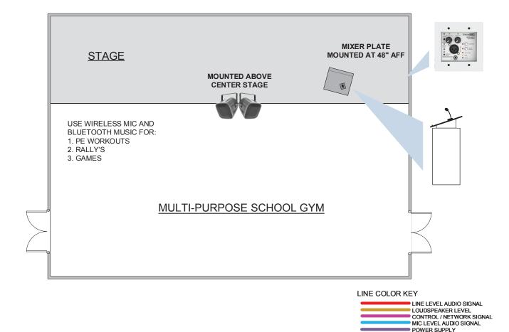
This is a design concept and is not meant to be a fully engineered system design. Contact AtlasIED for system design help.
