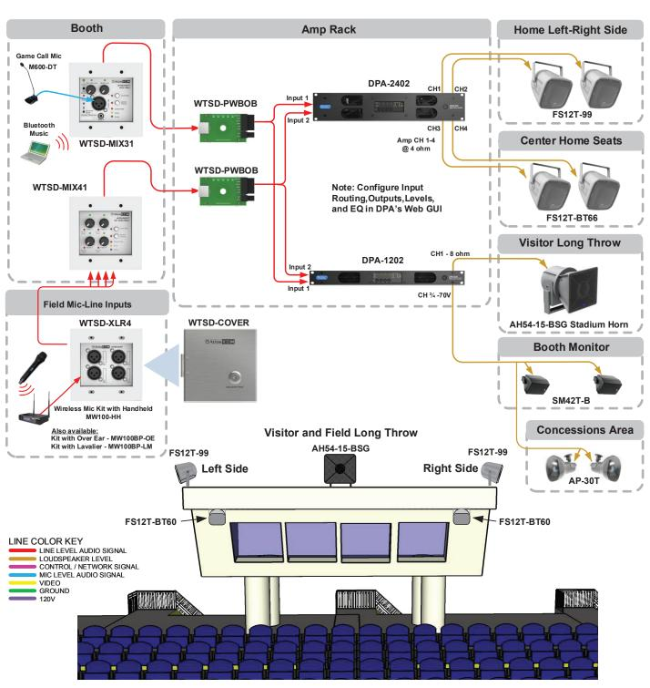
This is a design concept and is not meant to be a fully engineered system design. Contact AtlasIED for system design help.
