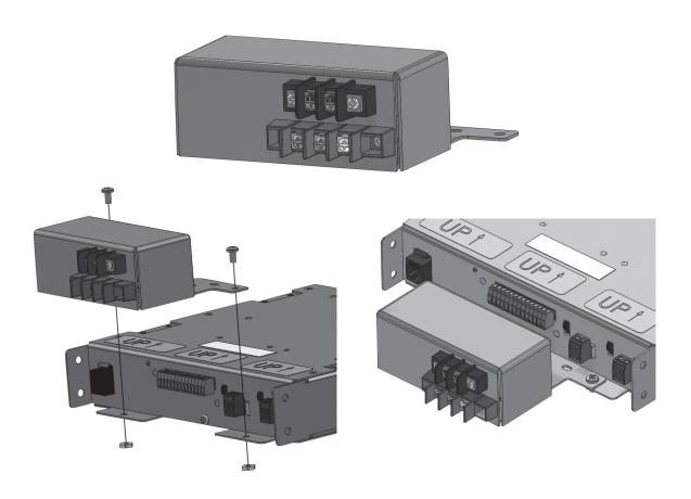
The ZCMT can be attached directly to the rear of the ZCM-V2+. Nuts and bolts included.
