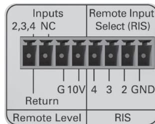
Connections to a 10K pot requires three conductors and a minimum of 22 gauge wire. The return ports can be paralleled together if one pot is to control all inputs. The AAPHD series remote level design is based on 10VDC return VCA type topology. Atlas Sound accessory level control WPD-RISRL can be used to achieve this.
