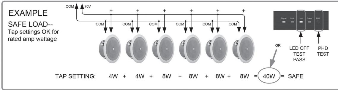
The Limit LED should never be constantly illuminated or damage may occur to the amplifier or sound system. If the Limit LED comes on steadily during use or during the PHD test there are a few common fault conditions to check if using a 70V distributed audio system.
