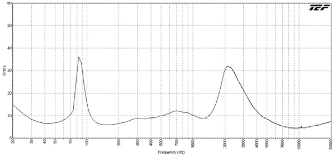
AH94-12T-BSG Impedance (Ohms) vs. Frequency
