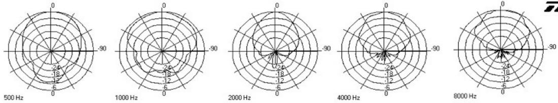
AH94-8T-BSG Horizontal Polars (Normalized To Zero On Axis) (-6dB)
