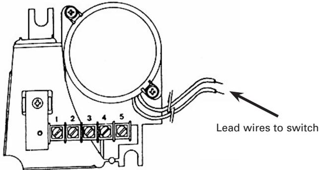
The WPVT-1S is an 8Ω, 15W intercom station employing a 2 point terminal strip for connecting to the 8Ω voice coil.
