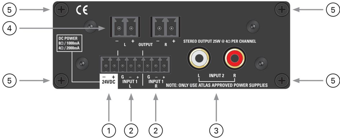
TSD Input/Output connections are removable for easy system wiring. The connectors have a 3.5mm pitch between pins.
