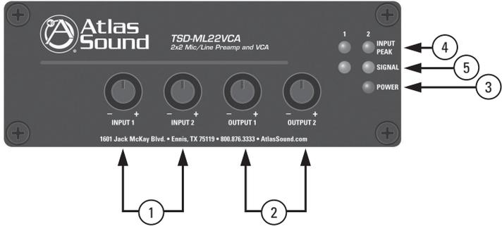
1. **Input 1-2 Level Controls** - Adjusts the gain of the independent input signals. Turn clockwise to increase the signal level and counter-clockwise to decrease it. **Note:** The Input Level Control knobs can be removed and replaced with a supplied security cover to prevent unauthorized adjustment.
