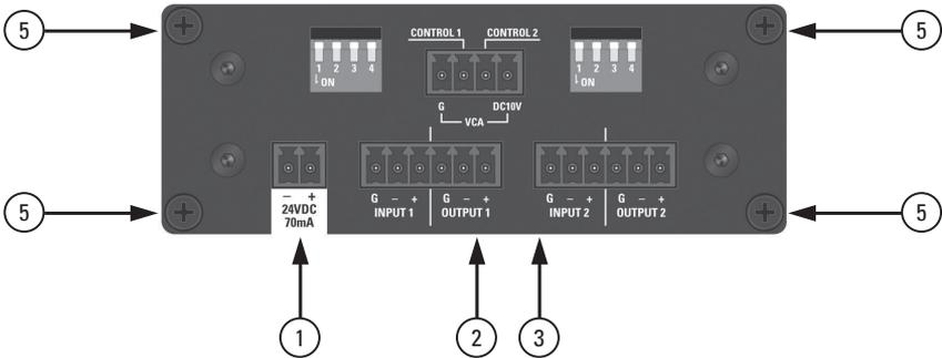
TSD Input/Output connections are removable for easy system wiring. The connector has a 3.5mm pitch between pins.
