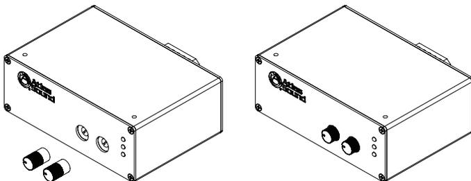
2. Security Cover Installation - Remove the knob from the panel and insert the cover. Small pliers may be required to remove the knobs. Align the security cover to the level control panel hole. Push the cover into the hole until it snaps into place. Do not force or damage may occur to the potentiometer.
