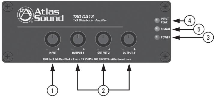
1. **Input Level Control** - Adjusts the gain of the source audio signal that is applied to the DA13 circuitry. Turn clockwise to increase the signal level and counter-clockwise to decrease it. **Note:** The Input Level Control knob can be removed and replaced with a supplied security cover to prevent unauthorized adjustment.
