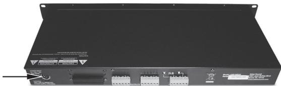
3. Remove 10 screws that secure the top cover. Note the screw types and placement for reinstalling the cover.
