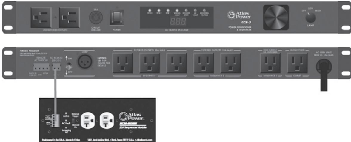
**ECM DCV Trigger** - The ECS-3 can handle 15A of current before the breaker opens. If 15A is not enough current to support your power requirements you can use the 24VDC trigger to activate an additional power outlet such as the ECM-20SH. This triggered 24VDC voltage works in conjunction with Sequence 3 timing section. Contact Atlas Sound for AC outlet options.
