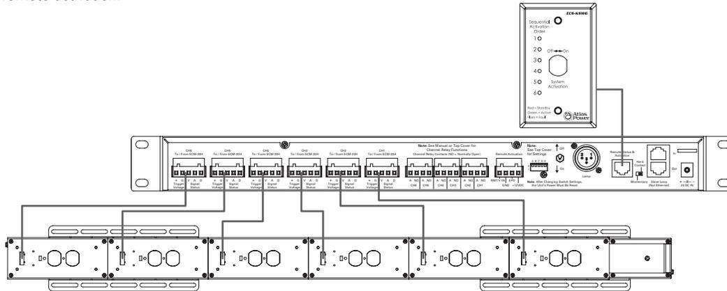
**Example 2:** 1 ECS-6RM<sup>B</sup> unit wired to 6 ECM-20 or ECM-20M modules in the ECM-RACEWY6 housing unit, using DCV 5-24V or a Switch for remote activation.
