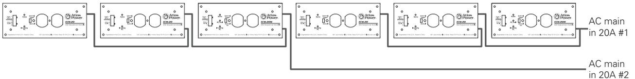
**Example 3:** ECM wiring configuration showing one 20A AC main line coming into 6 ECM-20M type modules. **Note:** It appears that the wiring is in series but the ECM Module In/Out terminals are in parallel on the PCB.
