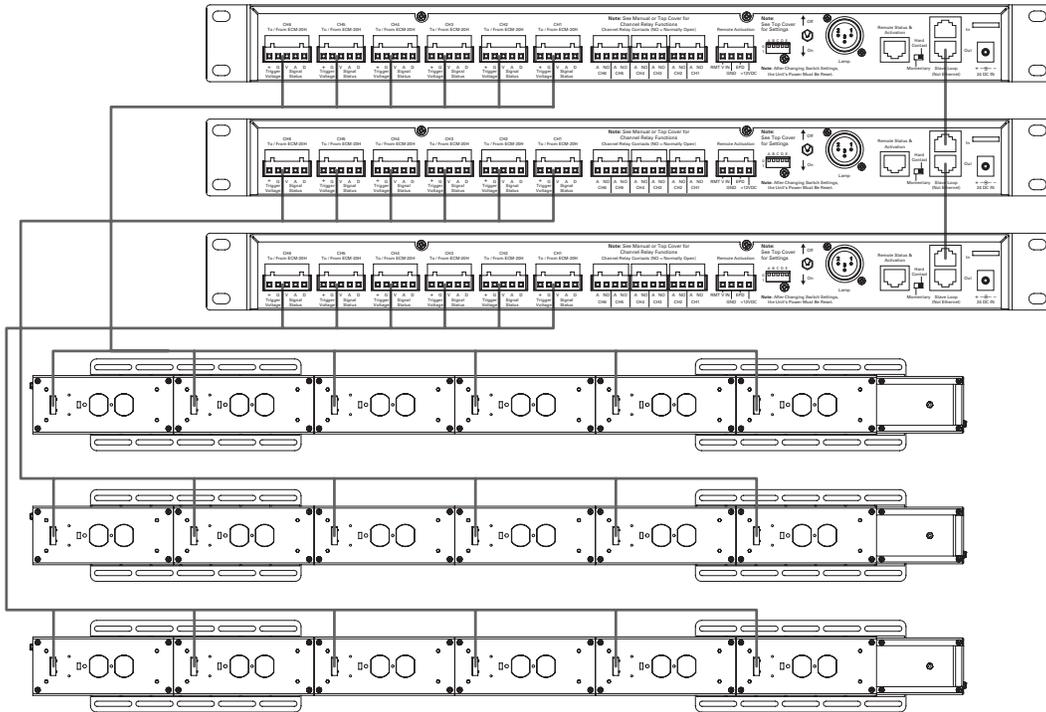
Example 4: 1 ECS-6RM<sup>B</sup> unit wired to 4 ECM-20 or ECM-20M modules in the ECM-RACEWY6 housing unit, and a separate ECM-15SH and ECM-20SH housing.
