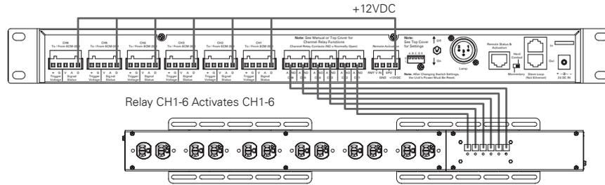
**Example 6:** Hybrid Design - 1 ECS-6RM<sup>B</sup> unit wired to 5 ECM-20 or ECM-20M modules in the ECM-RACEWY6 housing unit connected to CH1-5 Trigger Voltage / Signal Status inputs, and CH6 directly controlling 1 ESC-2063 module using one trigger contact from the ECS-6RM<sup>B</sup> to turn all 6 sections on at one time.
