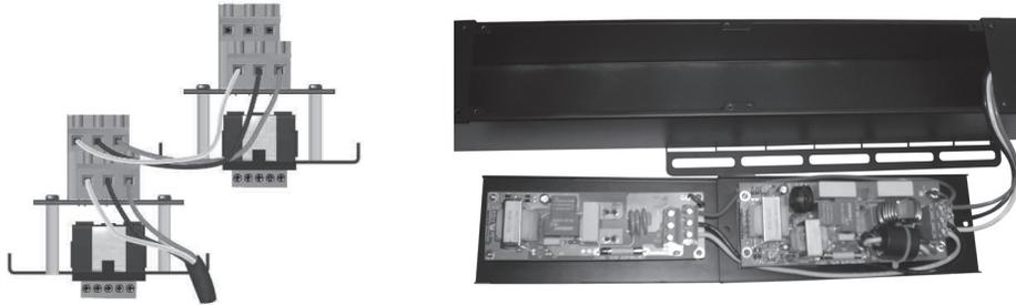
**Note:** The above figure shows the ECM wiring configuration of one 20A AC main line coming into an ECM-20M, then paralleling with an ECM-20 type module. It appears that the wiring is in series but the ECM Module In/Out terminals are in parallel on the PCB.
