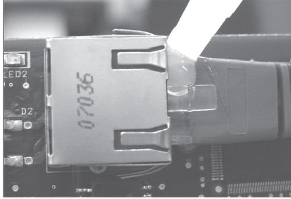
The electronic assembly within the IP-HVP is conformal coated to help protect against moisture. However, when installing outdoors, or in high moisture environments, it is essential that the RJ-45 network connector is completely sealed per the following instructions:
