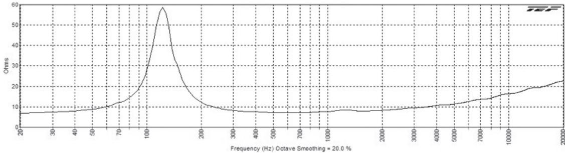
**FC104 Impedance (Ohms) vs. Frequency**
